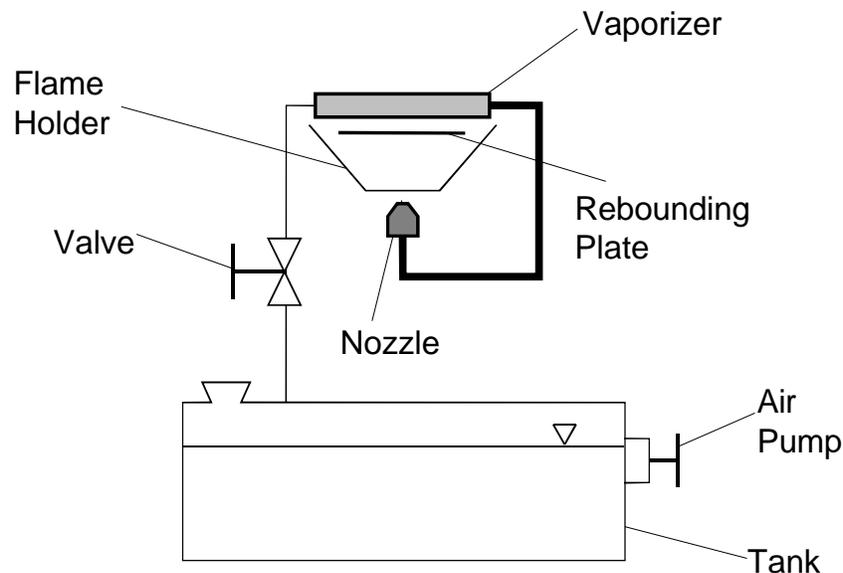
**Figure 1:** Function diagram of a pressure stove
